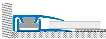
versatile and can be matched with all floor surfaces. Assemble with Clip CL 40 P + Aluminum base CLB 60 ANF.
