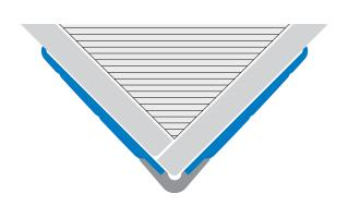
WALLPROTECTION WA 60 P\* Corner Guard in Solid Extruded Synthetic Resin This profile can be extruded in a single color or co-extruded for a "two-tone" design. The profile is tolerant to mechanical impact and most diluted chemicals and detergents. Available in white and grey. Other colors available upon request, minimum quantity required. See page 107.
