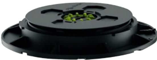
The Uptec SUPAL support is adjustable in height from 28 to 43 mm (1-3/32" to 1-11/16"), with a base with a diameter of 190 mm (7-31/64") and a head of 130 mm (5-1/8"). On the head it is possible to apply the accessories for standard installations (for 2 or 4mm joints; 5/64" or 5/32"), for laying with aluminum joist or for laying with wooden joist. Holes have been made on the base to allow the water to flow out, and on the lower side 4 pre-engraved lines for any cuts.
