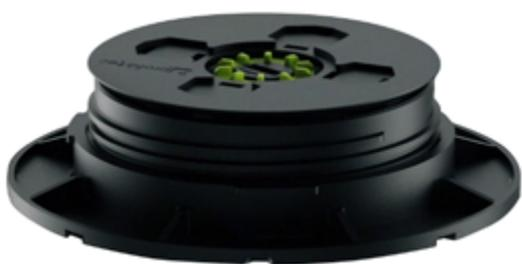
The Uptec SUPAS pedestal is adjustable in height from 43 to 58 mm (1-11/16" - 2-9/32"), with a base diameter of 190 mm (7-31/64") and a head of 130 mm (5-1/8"). On the head it is possible to apply the accessories for standard installations (for 2 or 4mm joints; 5/64" or 5/32"), for laying with aluminum joist or for laying with wooden joist. Holes have been made on the base to allow the water to flow out, and on the lower side 4 pre-engraved lines to cuts.
